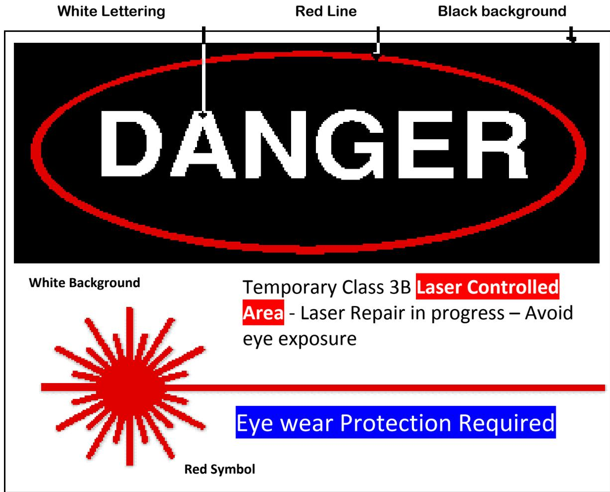
Figure 4 – Temporary Warning Sign requiring immediate hazard recognition
