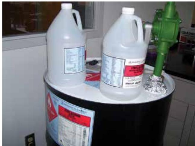
Excessive quantities of flammable liquids is a common violation cited during laboratory fire inspections.
