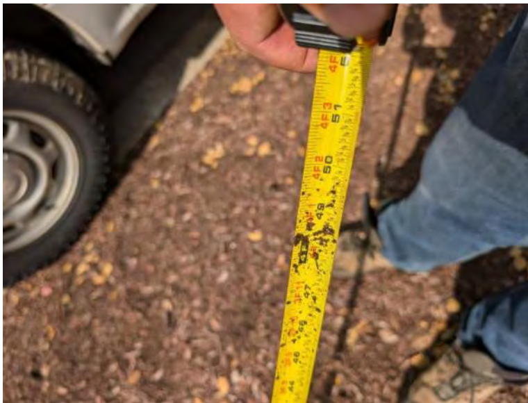
Measured 4ft of sediment accumulation
