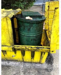
Containment not closed, spillage, no spill kit, no signage.
